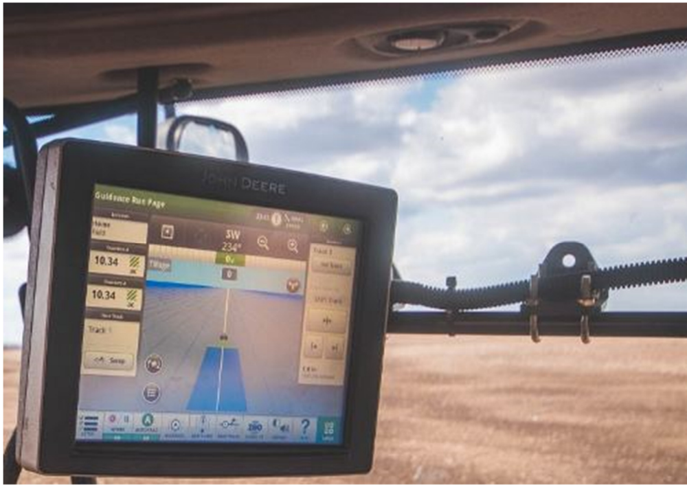
4640 installed at the top bar, cable coming from the opening in the back column.
