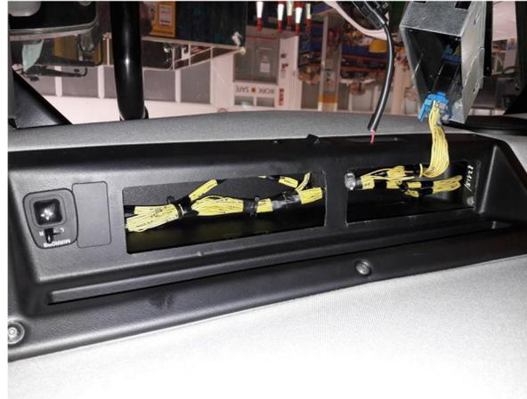
Locate the tractors radio antenna cable. Use the hole where this comes through and push the JD Antenna cable through this.
