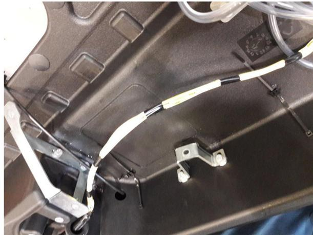
Locate the Front right-hand work light on the cab roof. Remove the whole work light assembly to gain access in the roof moulding. The JD antenna cable should be accessible.
