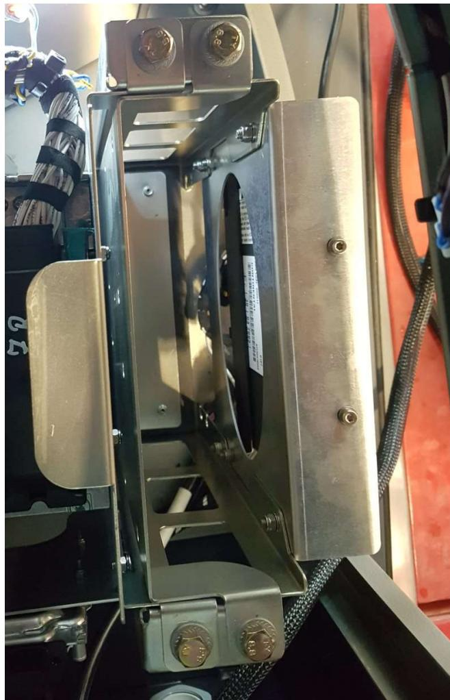
Bolt the Agra-GPS Horsch-JD Bridge with the cabling towards the bottom on the panel and slide it back in.
